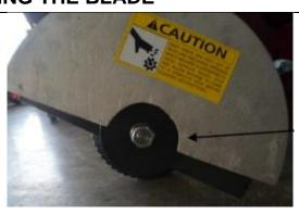
WARNING: Make sure the spark plug lead has been disconnected. Put a Stiltson on the pulley in the inside of the blade guard. Undo the bolt on the end of the drive shaft. It is best to use a air gun to remove this. Be careful the blade might rotate while loosening or tightening.
