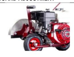
WARNING: Make sure the spark plug lead has been disconnected. The blade guard can position can easily be adjusted by loosening the bolt under the guard. Move it to the desired position and re-tighten. Do not over inflate the pneumatic wheel. Maximum PSI is 18.
