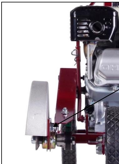
**WARNING: Make sure the spark plug lead has been disconnected.** Undo the two bolts on the blade flange. Pull the cutting head out so the belt is tight. Redo the bolts up. Do not over tighten drive belt
