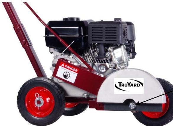
**WARNING: Make sure the spark plug lead has been disconnected.** Put a Stiltson on the pulley in the inside of the blade guard. Undo the bolt on the end of the drive shaft. It is best to use a air gun to remove this. Be careful the blade might rotate while loosening or tightening.
