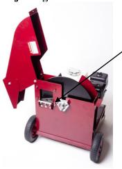
To adjust the anvil. Remove the discharge chute and the chipper chute. Loosen the three bolts on the underside of the anvil with a 13mm socket. Carefully move the anvil in your desired direction. For courser chips move away from the flywheel for finer chips move the nvil closer to the flywheel. With caution a move the flywheel around so the chipper blade is adjacent to the anvil and not touching.. When you tested both chipper blades distance redo the bolts up.
