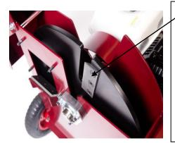
After time you will need to either replace the chipper blade or sharpen it. To remove the chipper blade you will firstly need to remove the chipper chute. You will now have access to the rear nuts on the chipper blades. You will need to remove these nuts with a 13mm Socket and an allen key to hold the screw. The blade will come out through the chipper chute entrance. When putting the blades back in you should always replace the bolts and nuts and lochtite the thread for safety.
